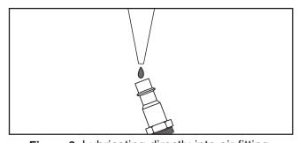
Figure 3. Lubricating directly into air fitting.
